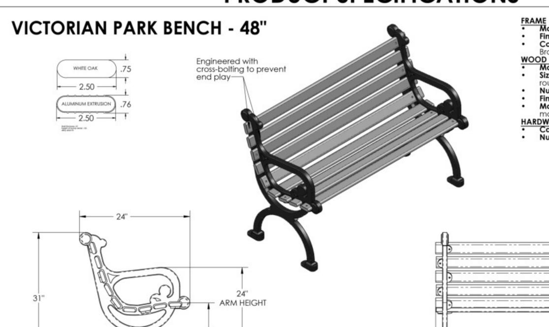
Material: Cast aluminum poured in permanent molds Finish: Electro static powder coating Color: Black, White, Green, Tan, Dk. Brown, Dk. Green, Bronze and Blue.
